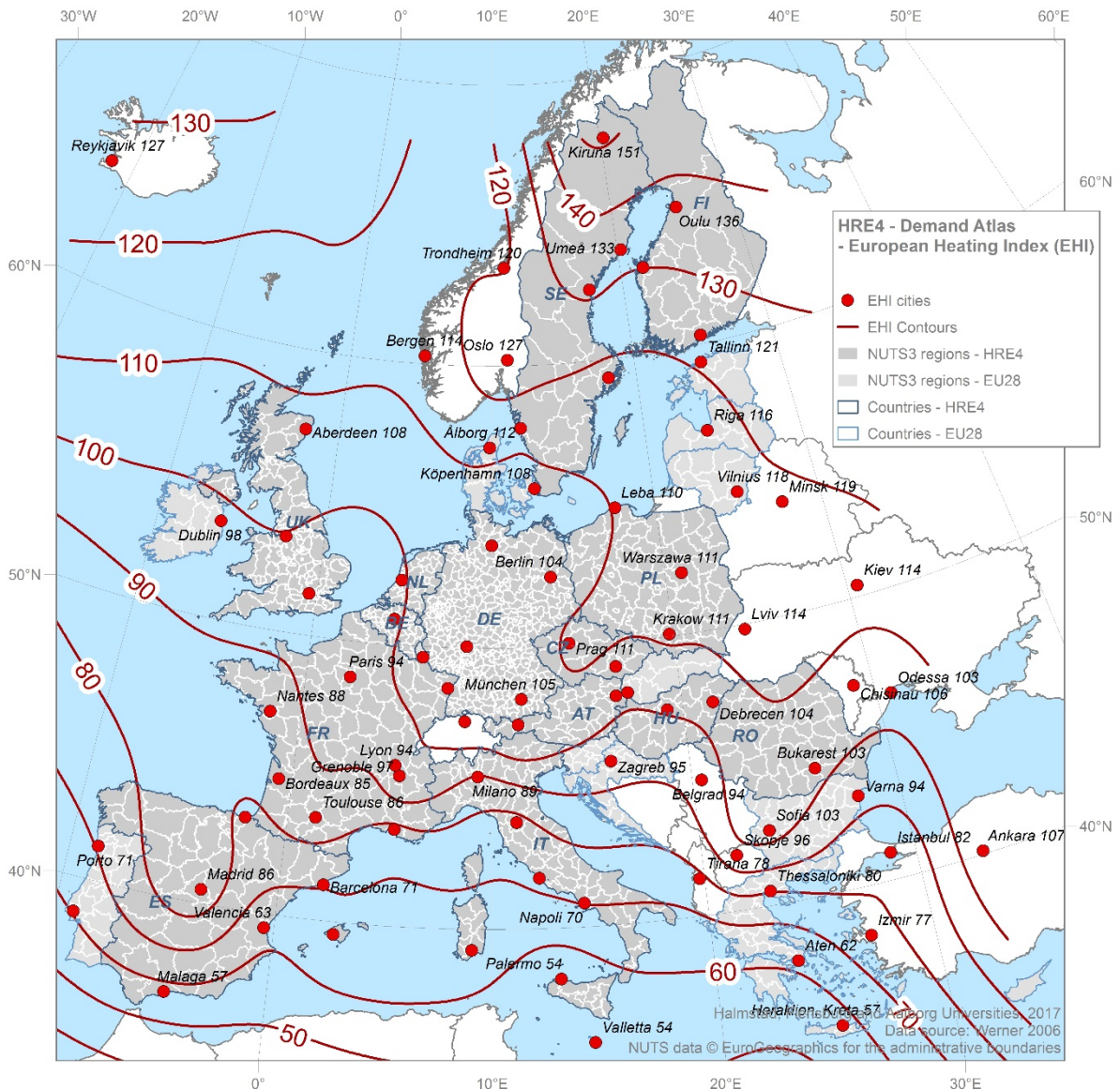
Figure 2.2. European Heating Index (EHI) values for 80 different locations in Europe and corresponding contour lines established by spatial interpolation. Sources: (Werner, 2006b, Werner, 2006a)
