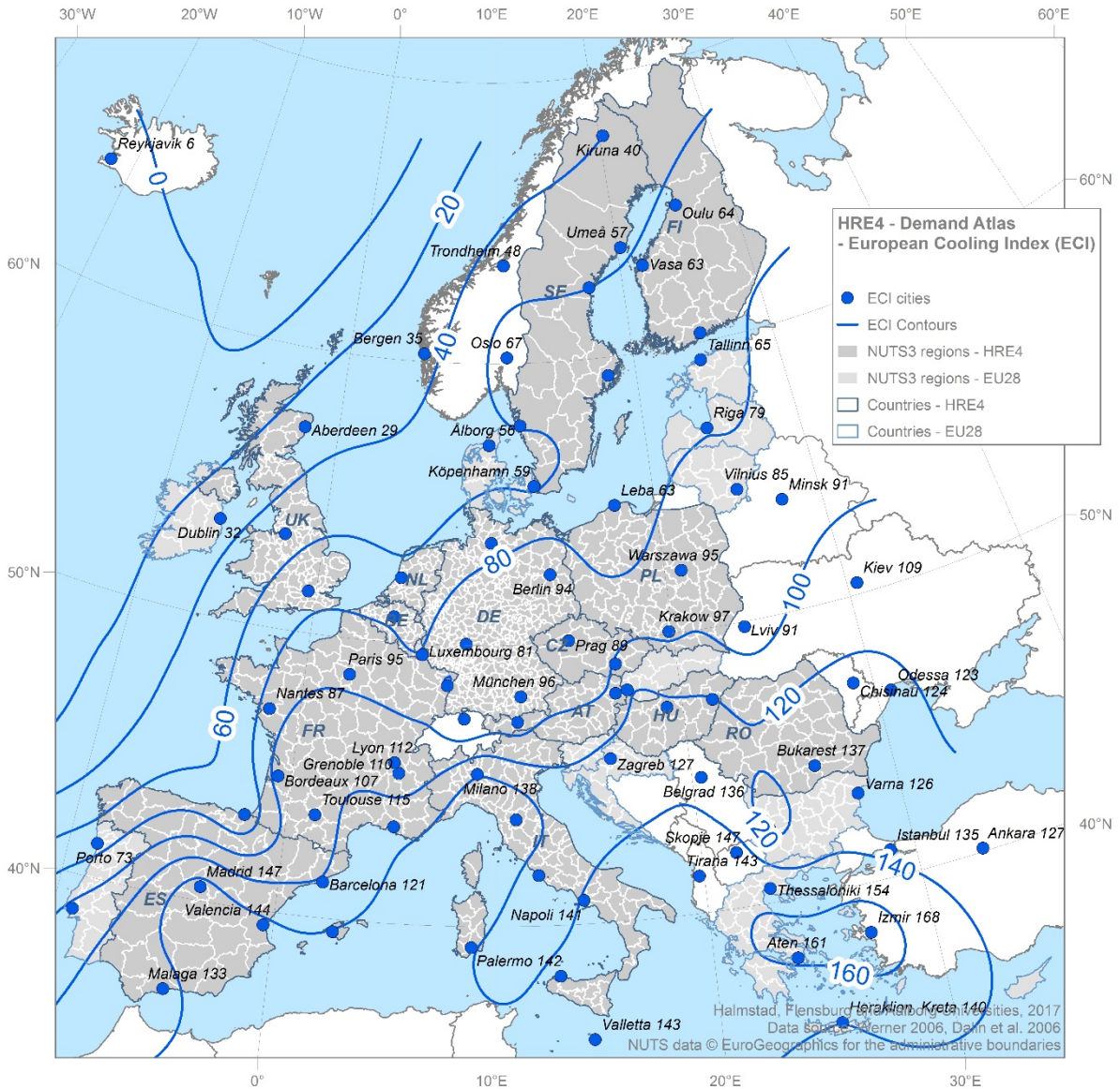
Figure 6.2. European Cooling Index (ECI) values for 80 different locations in Europe and corresponding contour lines established by spatial interpolation. Sources: (Dalin et al., 2005, Werner, 2006b)
