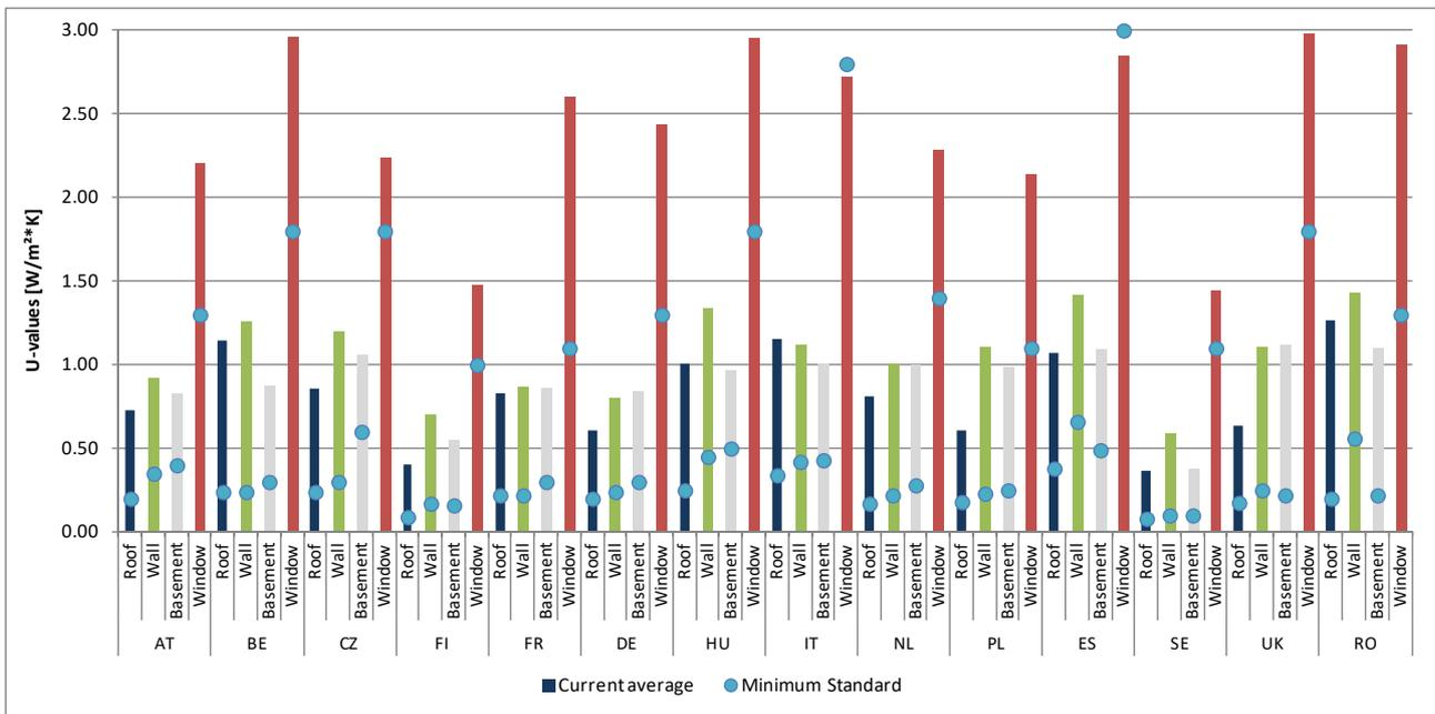
Figure 10: Current average building status (coloured bars) and future minimum standards (blue bullets, U-values in W/m²K) for the MFH building parts "wall", "window", "roof" and "basement".
