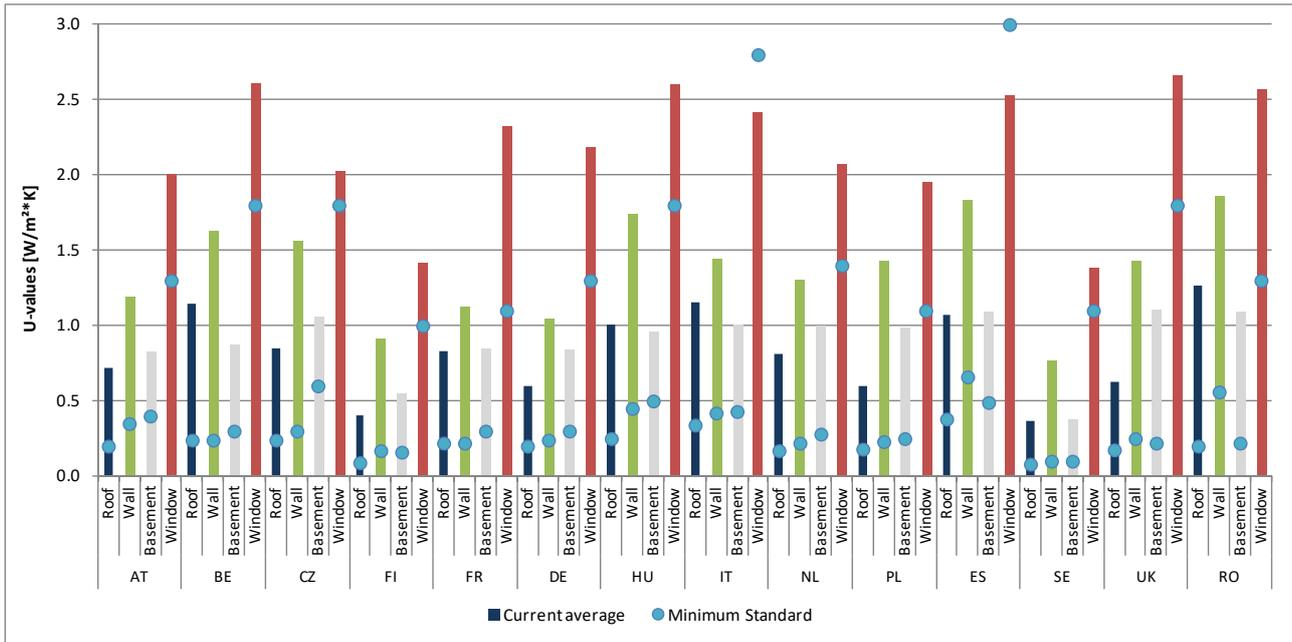
Figure 9: Current average building status (coloured bars) and future minimum standards (blue bullets, U-values in W/m²K) for the SFH building parts "wall", "window", "roof" and "basement".
