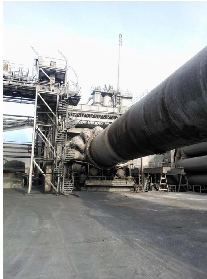
Rotary kiln (left) and plate heat exchanger (right) for recovery of flue gas excess heat to district heating at Portland Cement in Aalborg, Denmark. Photos: U. Persson.
